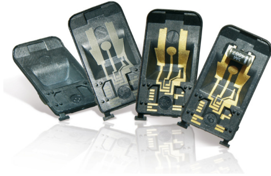
Fig. 1. Different fabrication steps of the LDS process - Injection molded, structured, metalized and assembled part
