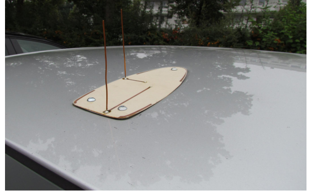
Fig. 6. (a) CAD model of the 2D reference monopole setup (3D antenna shown only as reference). (b) Picture of the reference 2D antenna mounted onto the sedan type vehicle used for measurement.
